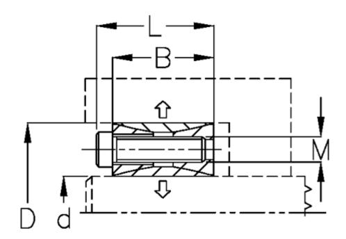
$\begin{array}{lll} \text{B mm} & = 20 \\ \text{d H8 mm} & = 19 \\ \text{D mm} & = 47 \\ \text{Fit tolerance} & = \text{Aksel k11-h11, Nav N11-H11} \\ \text{F kN torque} & = 17.0 \\ \text{L mm} & = 26 \\ \text{M mm} & = \text{M6} \\ \text{P N/mm2 surface pressure on shaft/hub} = 31 \\ \end{array}$
